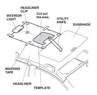
5. Using the utility knife, cut out the headliner around the edge of the template.
