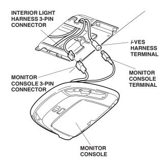
47. With an assistant holding the monitor console, secure the 3-pin connectors and terminals you plugged to the back of the monitor console.
