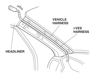
32. Continue routing the *i*-VES harness to the rear along the vehicle harness, and out of headliner opening you made, so that the distance between the headliner opening and *i*-VES harness terminal end is 14<sup>3</sup>/<sub>4</sub> in. (370 mm).
