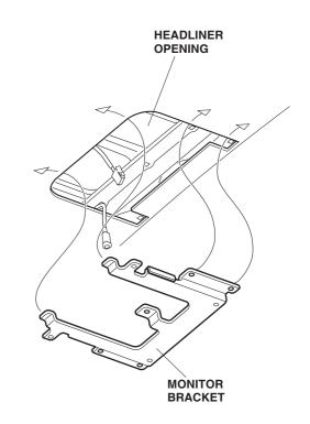
44. Install the monitor bracket to the vehicle frame with five square-neck bolts and five 4 mm flange nuts while holding the square-neck bolts.
