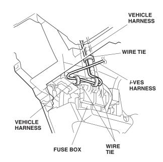
52. Continue to secure the *i*-VES harness to the vehicle harness with the three wire ties in the areas shown.
