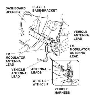
65. Wrap the FM modulator antenna lead and vehicle harness you removed with one wire tie with clip, and push the wire tie with clip into the hole in the player base-bracket.
