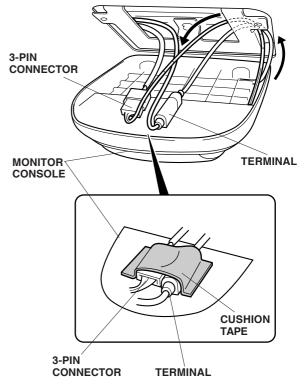
48. Secure the 3-pin connector and the terminal to the monitor console with one cushion tape.
