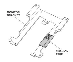
43. Insert the monitor bracket into the headliner opening.
