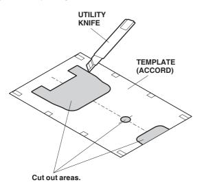
4. Close the sunshade. Position the template on the headliner align the interior light and headliner clip, and tape the template to the headliner using strips of masking tape.
