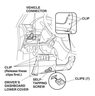
13. If equipped, remove the driver's dashboard under cover (release the three retaining clips, one pin and one holder).
