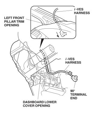
29. Continue routing the 90° end of the *i*-VES harness from the dashboard lower cover opening to the pocket opening on the driver's seat side.
