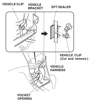
59. Using diagonal cutters, cut and remove the vehicle clip. Wrap one EPT sealer around the vehicle harness.
