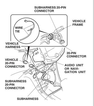
54. Secure the connected 20-pin connectors to the vehicle frame with two wire ties.
