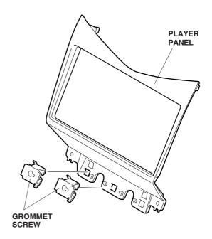
79. Insert the player panel clips into latches, and attach the player panel to the instrument panel with the two self-tapping screws removed in step 8. Remove the masking tape.
