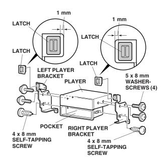
73. Position the DVD player and pocket on the left and right player brackets, and install four 5 x 8 mm washer-screws from the player kit, and the two 4 x 8 mm self-tapping screws from the player attachment kit. 74. Plug the subharness 4-pin connector, the DIN harness terminal and the *i*-VES harness terminal into the rear of the DVD player (plug the *i*-VES harness terminal into the yellow label position).
