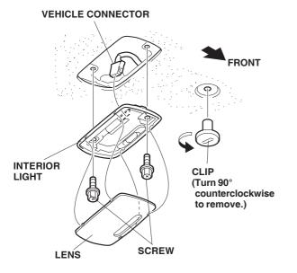
36. Remove the headliner clip by turning it 90° counterclockwise.
