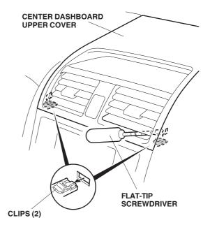
• Push the bottom of the hazard warning switch, and carefully insert a flat-tip screwdriver into the slot at the bottom of the hazard warning switch, then pry up the middle portion of upper panel by releasing the center clip.
