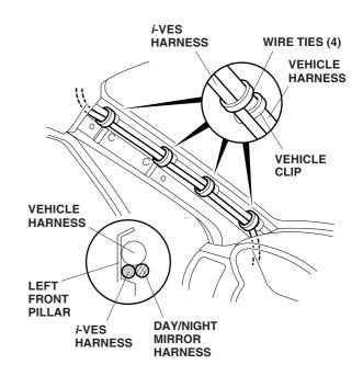
51. Near the fuse box by the dashboard lower cover opening, secure the *i*-VES harness to the vehicle harness with three wire ties in the areas shown.
