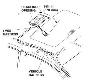
33. Using isopropyl alcohol on a shop towel, clean the area where the cushion tape will attach. Secure the *i*-VES harness to the underside of the vehicle frame with the two cushion tapes.
