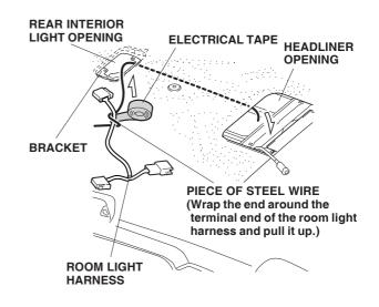
38. Wrap the end of the steel wire around the room light harness connector and secure with an electrical tape. Pull the room light harness up through the rear interior light opening and out through the headliner opening. 39. Plug the room light harness 3-pin connectors in between the rear interior light and vehicle 3-pin connectors and wrap one EPT sealer around the 3-pin connectors.
