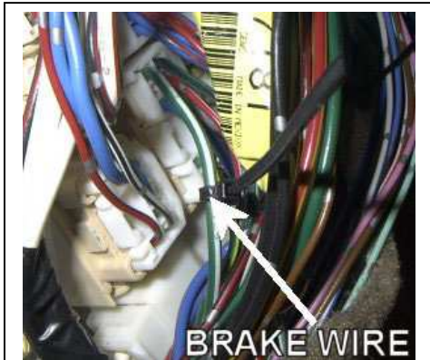
Location of the brake wire in the driver's kick panel of a 1999 Toyota Avalon.
