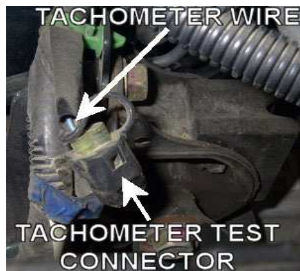
Tach location near battery for 98-02 Honda Accord 4-cylinder
