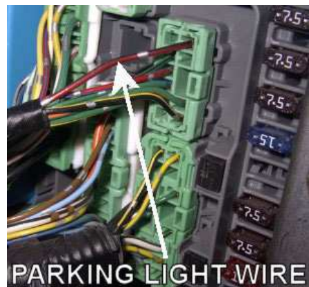
Pictured is the location of the parking light wire at the driver's side fuse box for 1998-2002 Honda Accords. On almost all Hondas and Acuras, the parking light wire can be found at the fuse box.
