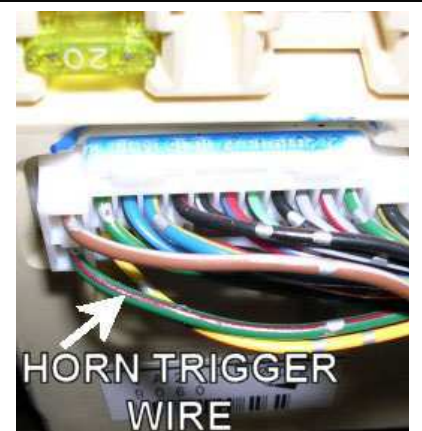
The location of the horn trigger wire at the fusebox of a 2001 Toyota 4Runner.
