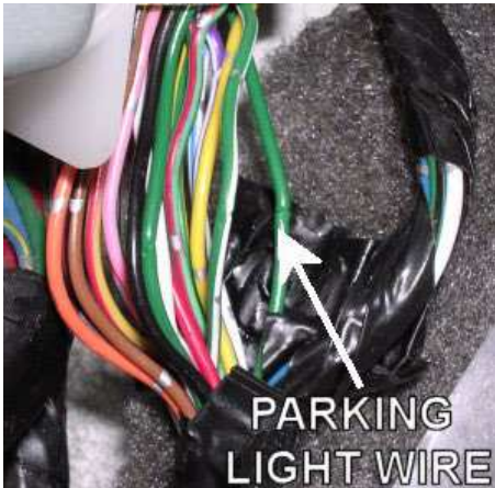
Pictured is the location of the parking light wire in a harness running towards the rear of the vehicle in a 2001 Toyota 4Runner.
