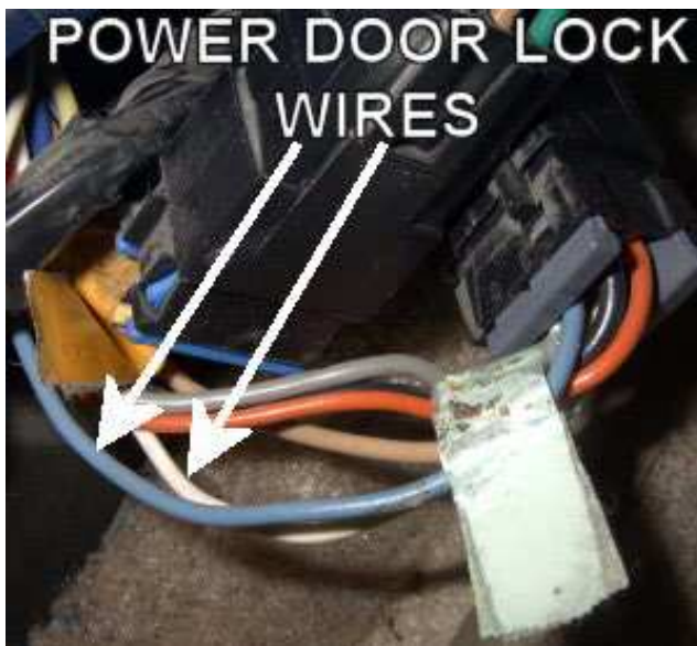
Pictured is the location of the power door lock wires in the driver's kick panel of a 1998 Chevy Suburban.
