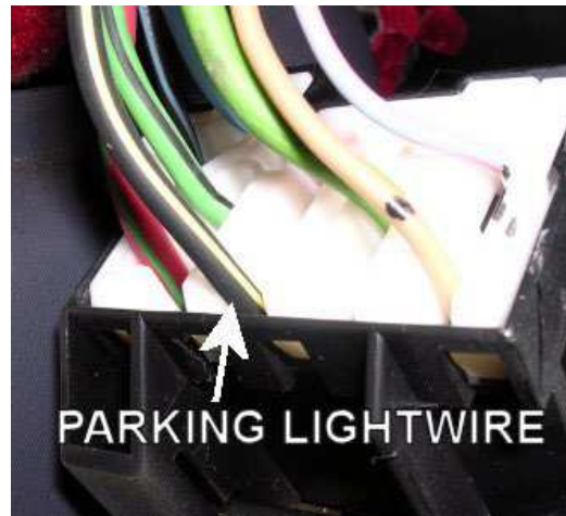
On many vehicles, the parking light wire can be found behind the headlight switch. (ABOVE LEFT) Pictured is the location of the parking light wire in the connector that plugs into the headlight switch of a 1998 Chevy Suburban. This location will be similar in 1998-2000 GM Full Size Pickups and SUVs. (ABOVE RIGHT) Pictured is the location of the parking light wire behind the headlight switch of a 1998 Dodge Durango.
