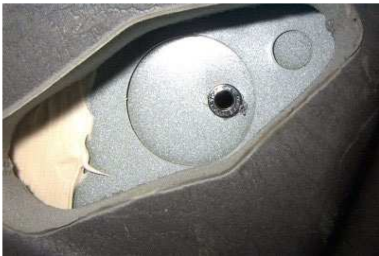
The picture above shows that a hole was drilled in the spot where the clutch cable would go through the firewall. The hole was drilled using a unibit.
