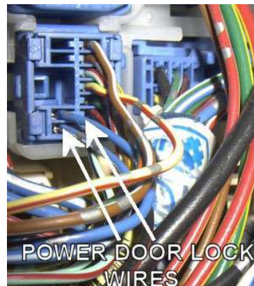
On a 1999 Toyota Avalon, the power door lock wires are in the passenger kick panel but can also be found in the driver's kick panel. Test by using the key in the driver's door. Unlock requires a double pulse
