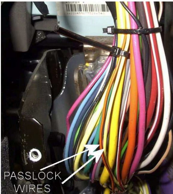
(LEFT) Shown is the location of the Passlock II wires (18 gauge YELLOW and ORANGE/BLACK) in the ignition harness of a 1998 Chevy Suburban. 1998-2002 Chevy and GMC full-size trucks and SUVs will be similar. BE CAREFUL WORKING AROUND AIRBAG WIRES, which can be found in yellow split loom or tubing in the ignition harness.
