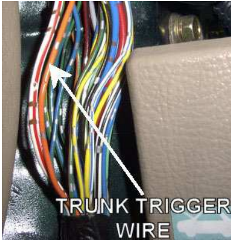
This picture shows the location of the trunk trigger wire in a harness in the driver's kick panel leading towards the rear of the vehicle of a 2000 Honda Accord.
