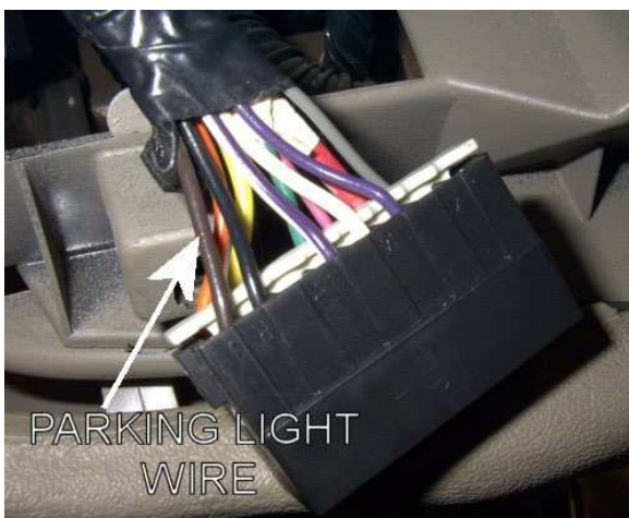
On many vehicles, the parking light wire can be found behind the headlight switch. (ABOVE LEFT) Pictured is the location of the parking light wire in the connector that plugs into the headlight switch of a 1998 Chevy Suburban. This location will be similar in 1998-2000 GM Full Size Pickups and SUVs. (ABOVE RIGHT) Pictured is the location of the parking light wire behind the headlight switch of a 1998 Dodge Durango.
