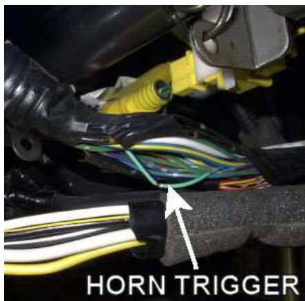
The location of the horn trigger wire in the ignition harness of a 1999 Honda Accord.
