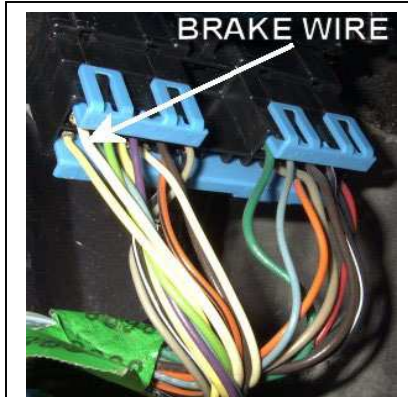
Location of the brake wire at the driver's kickpanel of a 1996 Chevy Cavalier.
