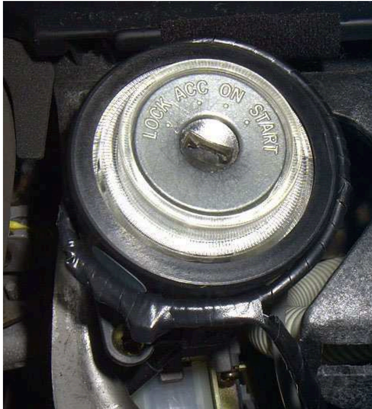
Example of the Immobilizer bypass module's antenna ring placed around the vehicle's ignition key cylinder.
