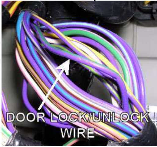
Door lock/unlock wire of a 2001 Dodge Caravan.
