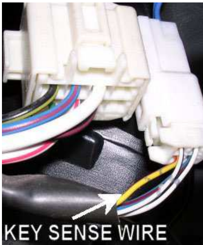
Pictured above is the location of the key sense wire in a small connector by the ignition key cylinder on a 2001 Toyota 4Runner. On most vehicles, the key sense wire can be found in a small connector near the vehicle's ignition cylinder.
