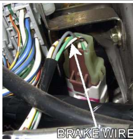
Location of the brake wire at the brake pedal switch of a 1998 Honda Accord EX.
