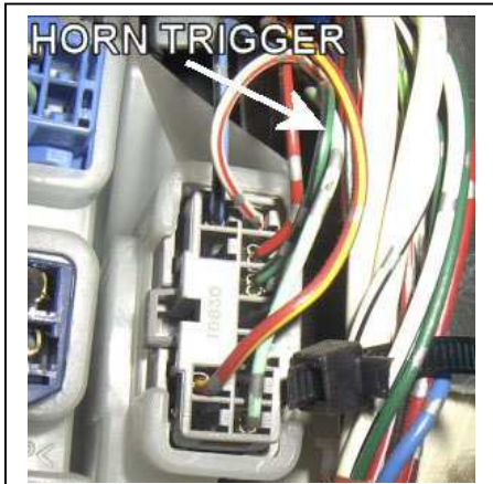
The location of the horn trigger wire in the driver's kickpanel of a 1999 Toyota Avalon.
