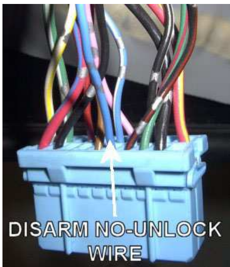
The shows the location of the factory alarm disarm-no-unlock wire in the harness at the driver's window switch of a 1999 Honda Accord EX.
