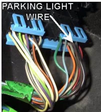
Pictured is the location of the parking light wire in the black connector in the driver's kick panel of a 1997 Pontiac Sunfire.
