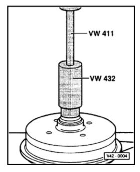
Fig. 6 Outer wheel bearing outer race, pressing in
