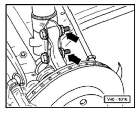
Fig. 2 Wheel bearing housing/suspension strut joint, separating
