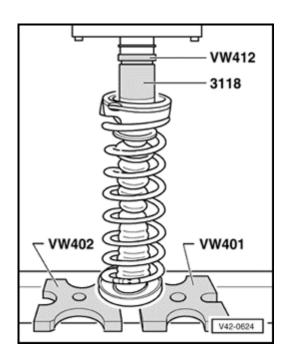
Fig. 5 Cap, pressing into suspension strut mounting
