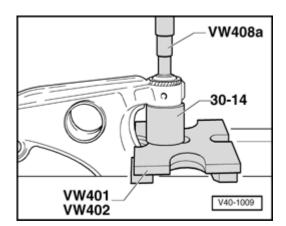
Fig. 1 Front control arm mounting, pressing out
