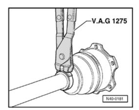
Tighten small diameter clamp with VAG 1275 pliers or equivalent (e.g. KD 474).
