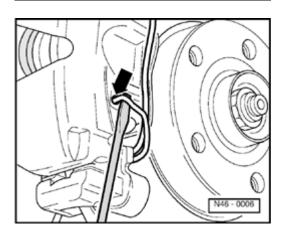
Pry off brake pad retaining spring from brake caliper housing with a screwdriver and remove.
