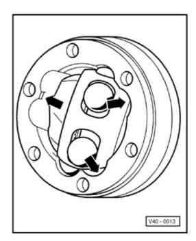
Swivel in ball hub, whereby the hub must be swivelled out of the cage (arrows) far enough to allow the balls to fit into the ball tracks.
