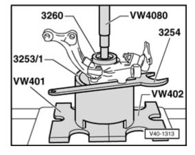
Fig. 4 Wheel bearing, pressing out of wheel bearing housing
