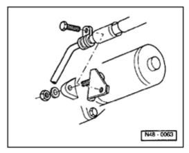
Fig. 2 Pressure hose, securing (vehicles with automatic transmission)
