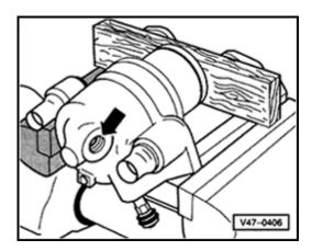
Fig. 1 Piston, pressing out of cylinder using compressed air
