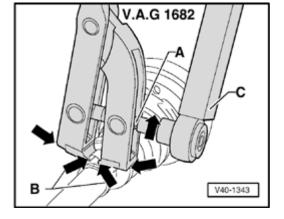
Fig. 3 Tightening small end clamp
