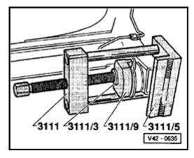
Fig. 8 Rubber bonded mounting, presssing into axle beam
