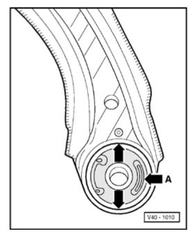
Fig. 2 Control arm rear mounting, installation position
