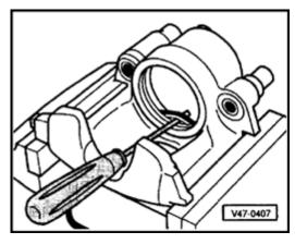
Fig. 2 Piston seal, removing
