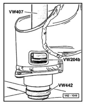
Fig. 4 Wheel bearing, pressing in
