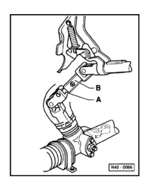
Universal joint shaft 25 Nm (18 ft lb) halves
