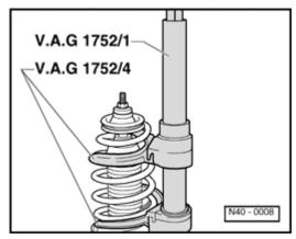
Fig. 2 Spring, removing and installing
