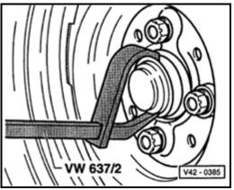
Fig. 2 Grease cap, pressing off
