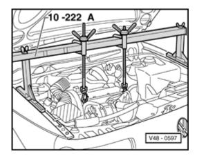
Fig. 5 Supporting engine/transmission assembly with 10-222 A and legs 10-222 A/1
