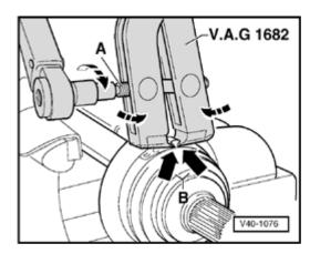
Fig. 2 Tightening outer CV joint boot clamp
