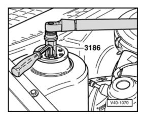
Fig. 1 Suspension strut to body, loosening and tightening
