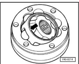
Swivel in the hub with balls by applying firm pressure on the cage (arrow).
