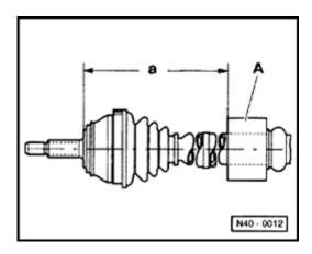
When installing vibration damper -A- note correct installation position. Ensure dimension "a" is maintained.
