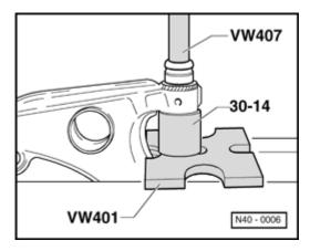
Fig. 2 Front control arm mounting, pressing in
