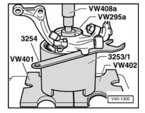
Fig. 2 Hub, pressing out of wheel bearing housing
