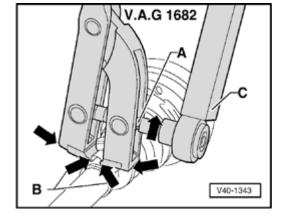
Fig. 4 Clamp, tightening on small diameter
