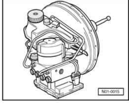
✓ The ABS hydraulic unit -a- and ABS control module -b- together make up one component. Separating them for service is only possible after the assembly has been removed.
