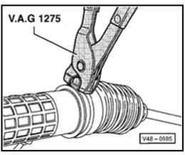
Tension hose clamps with pliers VAG 1275 or equivalent.
