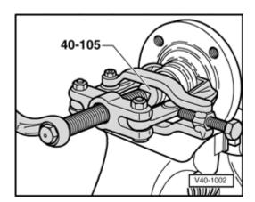
Fig. 3 Inner race, pulling off hub
