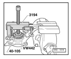
Fig. 6 Wheel bearing, pressing out of wheel bearing housing
