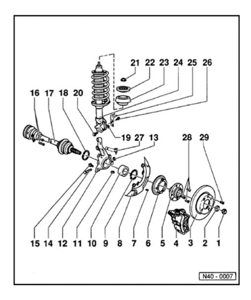
Wheel bearing, suspension strut and drive shaft, removing and installing (Base running gear)
