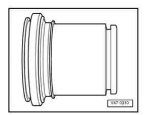
Fig. 3 Protective seal, installing
