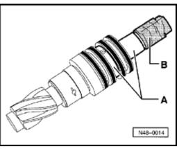
Tape the valve body with adhesive tape.
