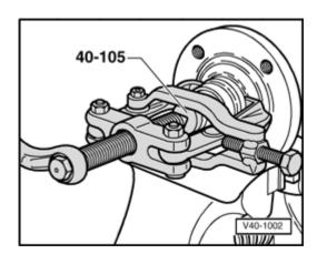
Fig. 5 Bearing race, pulling out of hub
