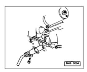
Fig. 1 Pressure hose, securing (vehicles with manual transmission)
