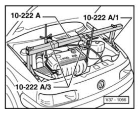
Fig. 4 Engine/transmission assembly, supporting with 10-222 A and 10-222 A/3
