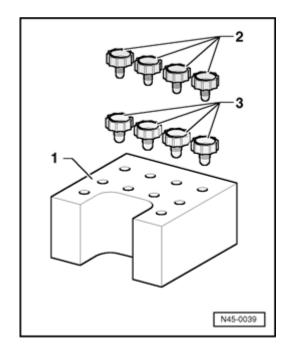
After separating ABS control module from ABS hydraulic unit, always install valve dome transportation protection on hydraulic unit.
