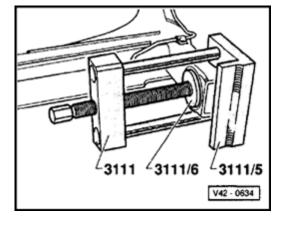
∢ Fig. 5 Bonded rubber mounting, pressing 1st half out of axle beam
