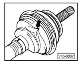
Fig. 7 Joint boot, ventilating
