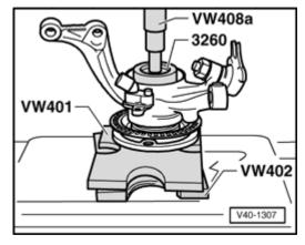
Fig. 6 Hub, pressing into wheel bearing housing
