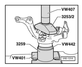
Fig. 5 Wheel bearing, pressing into wheel bearing housing
