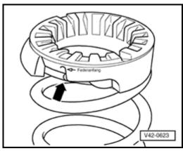
Fig. 2 Spring seat, installation position
