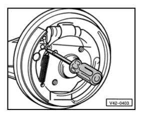
Fig. 5 Brake shoe adjustment, releasing
