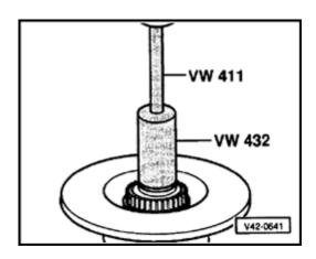
Fig. 7 Inner wheel bearing outer race, pressing in
