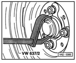
Fig. 2 Grease cap, pressing off
