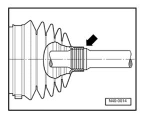
Fig. 10 Installation position of left drive shaft wheel end joint boot, shaft diameter 27 mm
