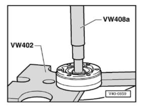
Fig. 3 Inner constant velocity joint, pressing off
