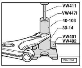
Fig. 4 Control arm rear mounting, pressing out and in
