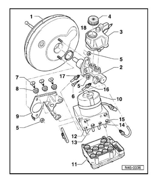
ABS, ABS/EDL hydraulic unit, vacuum brake booster and brake master cylinder (Teves 20 GI), servicing
