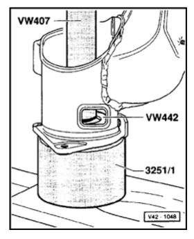
Fig. 2 Wheel bearing, pressing out
