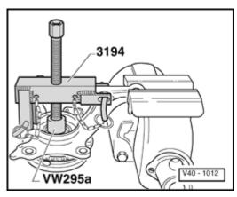
Fig. 3 Ball joint/control arm connection, separating
