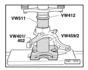
Fig. 7 Wheel bearing, pressing into wheel bearing housing
