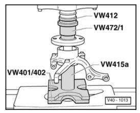
Fig. 8 Hub, pressing into wheel bearing housing
