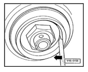
∢ Fig. 3 Grease cap, driving on
