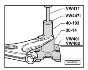
Fig. 3 Control arm rear mounting, pressing out and in
